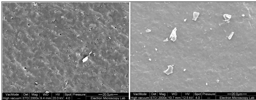
Figure 8: 2000x SE fracture surface images for sintered samples – (left): HS and (right): LTS B 4 C – 20 µm scale bar
