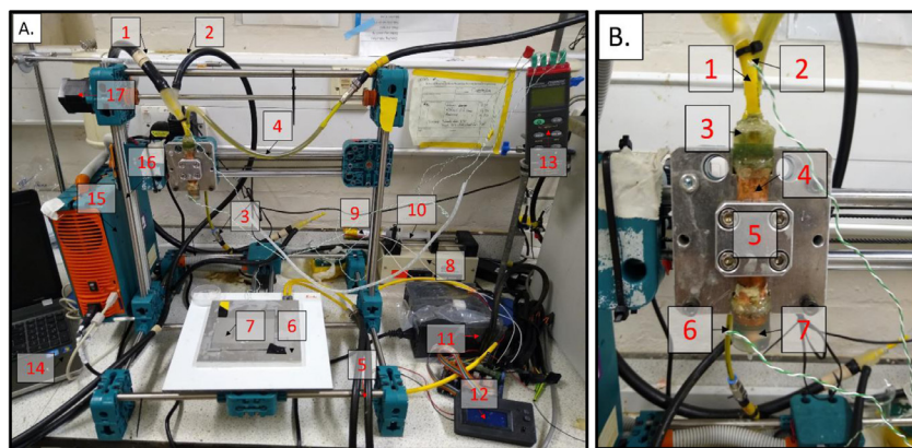
in place, (6) Thermocouple to monitor temperature of feed material as it enters the die, (7) 3D Printed nozzle. The printer was connected to and controlled by a computer running Netfabb for Fabbster software.
