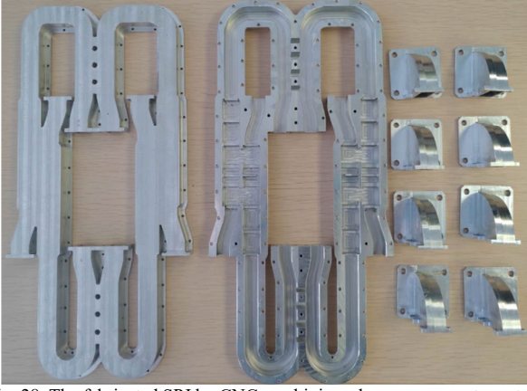
Fig. 28. The fabricated SPJ by CNC machining, shown as separate parts.
