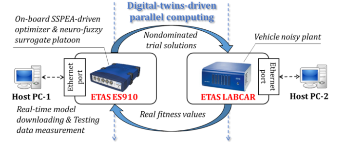
Fig. 6. Hardware-in-the-loop testing bench
