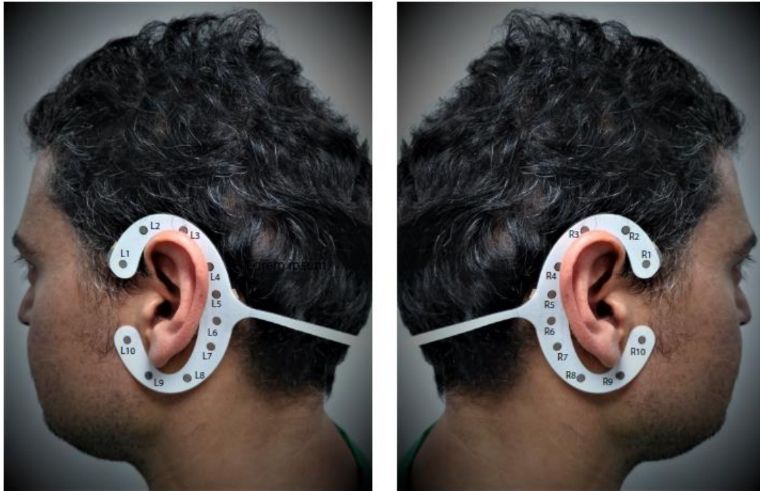
Figure 1. Layout of the cEEGrid electrodes. The right mastoid (R5) served as the ground while the left mastoid (L6) served as the reference during the online recordings. The data were offline re-referenced to a linked mastoid where L6 and R6 served as the reference.
