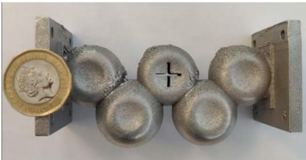
FIGURE 20 Photograph of the selective laser melting printed Filter UDS2
