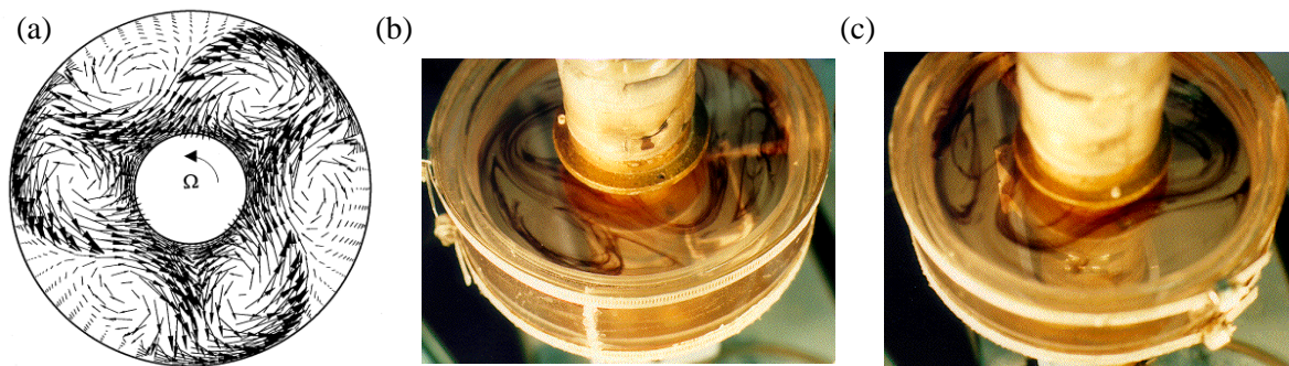
Figure 18. Idealized atmospheric jet stream with three cyclones and three anticyclones (from Tucker [28])
