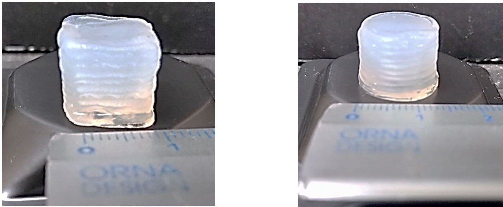
403 Figure 5: 3D printed 12 mm cube (A) and 12 mm height and diameter cylinder (B) printed using 3% κC and 2% 404 thiamine hydrogel
