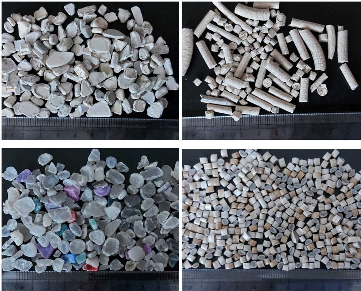
Figure S3: Colour sorted MEP chips and pellets. Clockwise from the top left: “white” sorted MEP chips; extruded “white” MEP pellets; extruded “clear” MEP pellets; “clear” sorted MEP chips.
