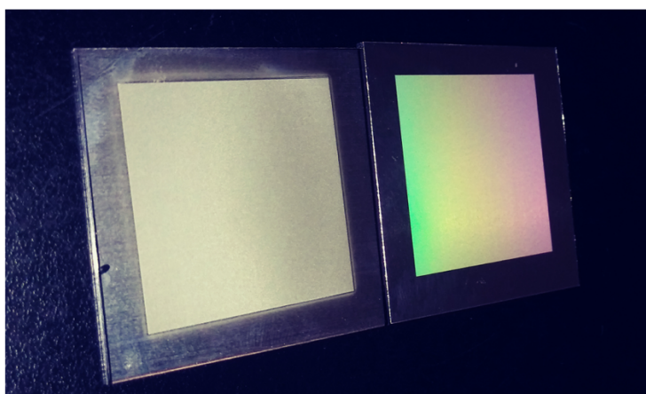
Figure S1: Optical images of femtosecond laser-induced multiscale (left) and LIPSS (right) topographies on SS. Processed area is 30 mm x 30 mm.
