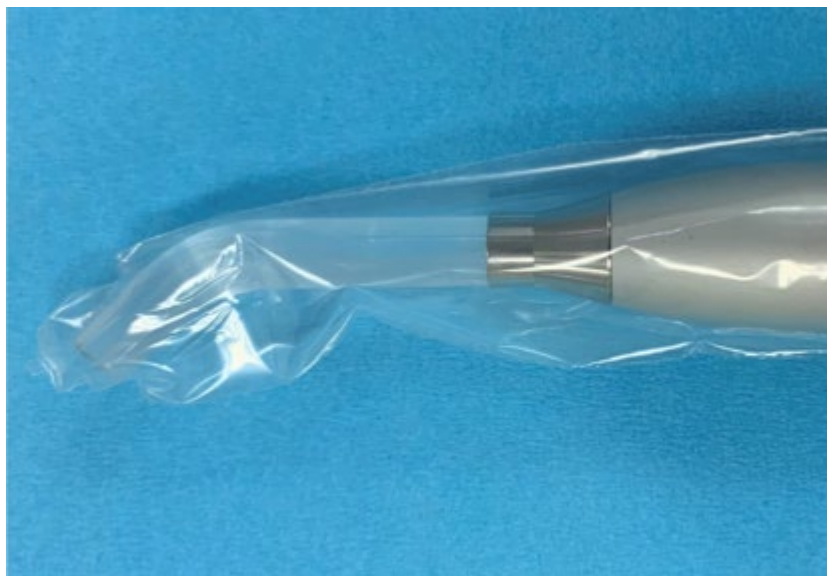
Figure 1: Satelec mini LED (Acteon, Merignac, France) with a light protective sleeve (WRAPAROUND, UnoDent, Essex, England) over the tip.
