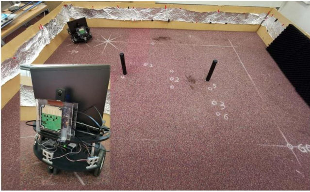
FIGURE 8 Photo of the robot and its working space with two cylindrical obstacles
