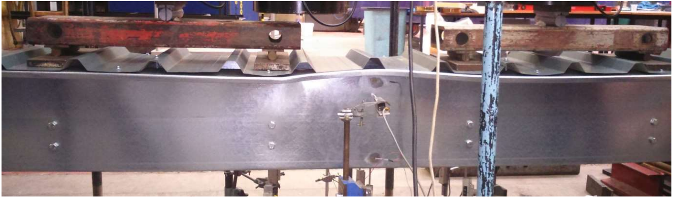
Fig.14: Failure mode of Z30718 - distortional buckling and localization of failure at left loading point (i.e. web crippling) after the peak load.
