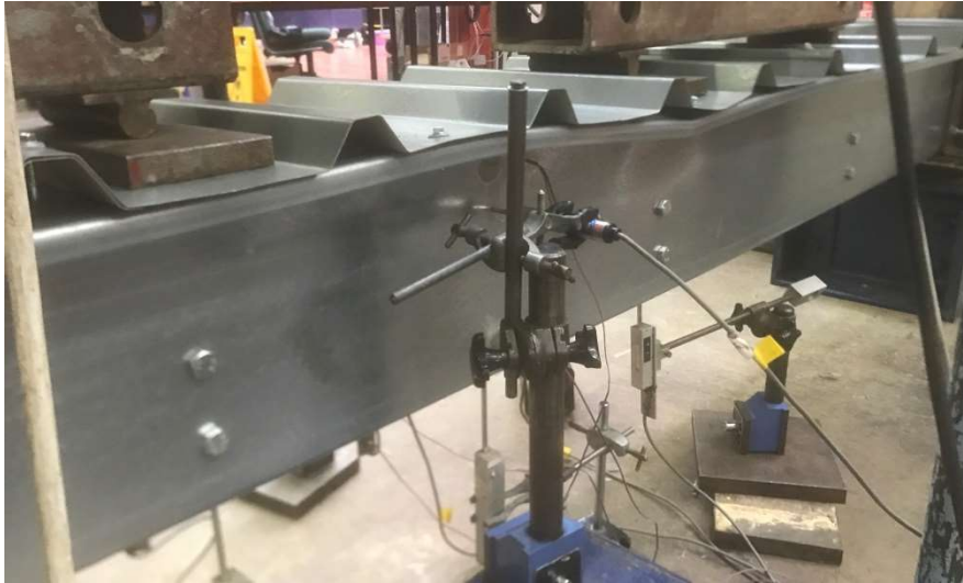
Fig.13: Failure mode of Z24620 - distortional buckling.
