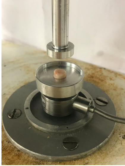
Figure 3: Experimental setup for the compressive DMA of brain tissue specimens.
