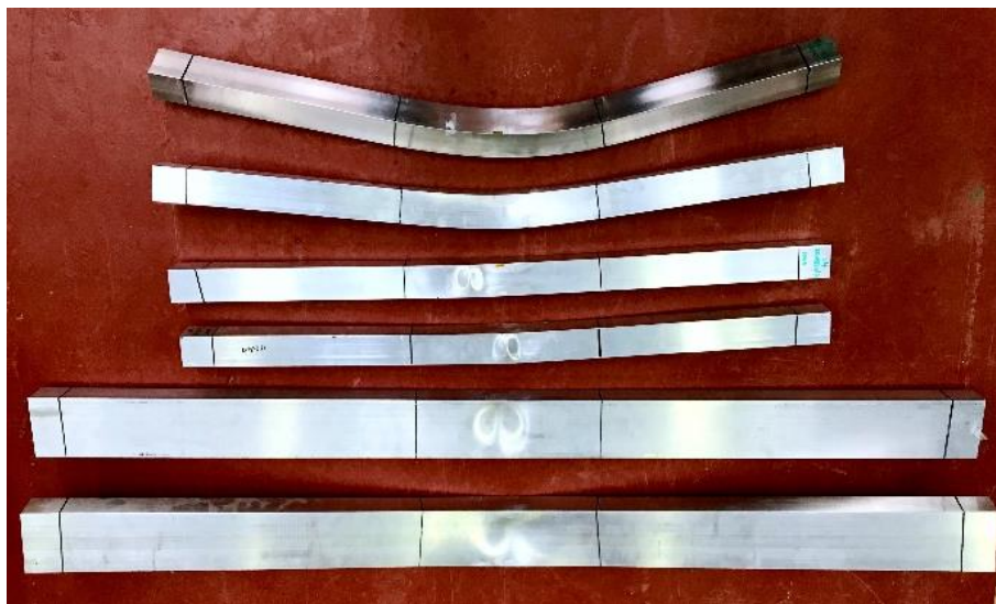
Figure 10 Failed beams subjected to biaxial bending
