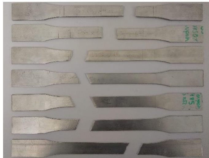
Figure 2 Failed tensile coupons
