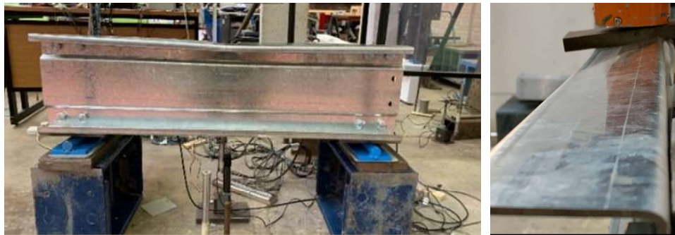
Fig. 7. Web crippling of the upper web of specimen 26525-50
