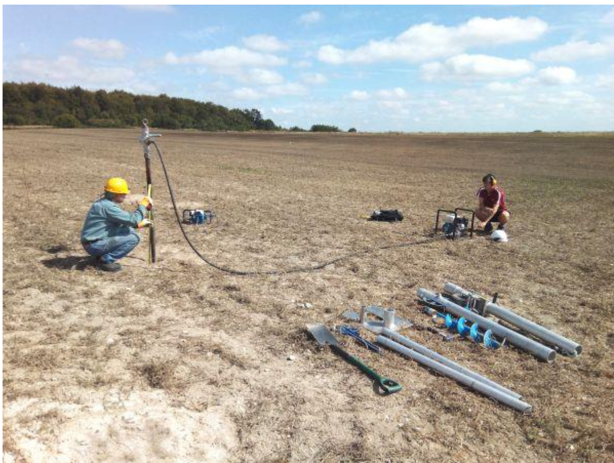
Figure 11: Vibracoring at 8A, looking north-east towards Durrington Walls
